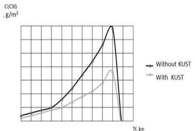
**Figure 6. Dependence of hydrocarbon concentration in the exhaust gas on engine power**
