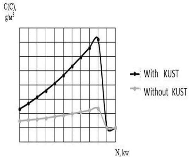
**Figure 7. The dependence of the concentration of soot in the exhaust gas from the load of the engine**
