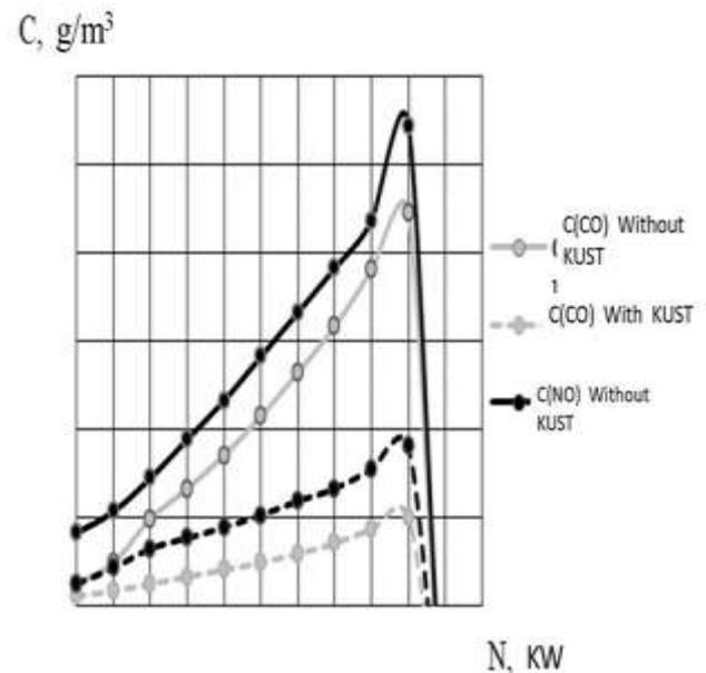
**Figure 5. Dependence of CO and NOx concentrations in the exhaust gas on engine power**
