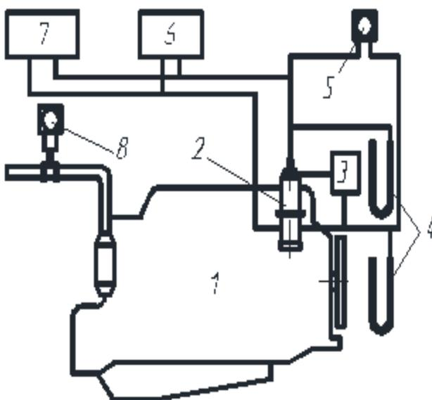
1 - engine YMZ-238; 2 - experimental KUST; 3 - temperature meter ITP-2; 4 - piezometers; 5 - exhaust gas flow meter; 6 - TESTO-350 gas analyzer; 7 - Infrakar 1 smoke meter; 8 - fuel meter "Port-1"
