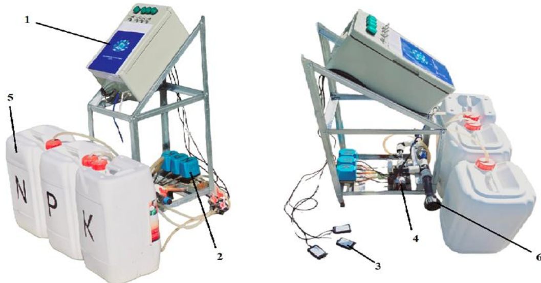
Figure 2. Fertilization unit in the automated and semi-automated irrigation fertilization system
