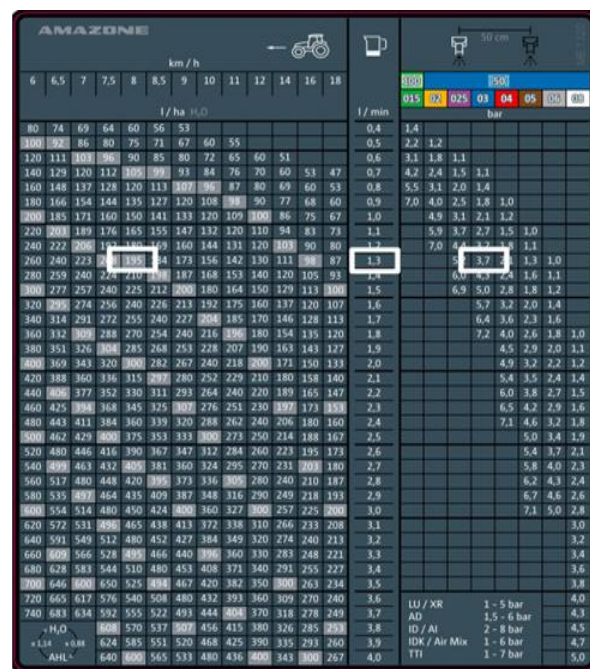
Figure 4. Sprayer adjustment nomogram
