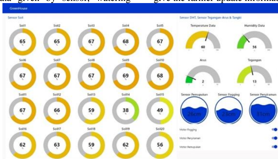
Fig. 9. IoT monitoring interface for the agrivoltaic system
