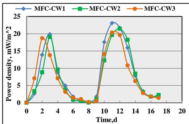
**Figure 2. Profiles of power generation in MFC-CWs**
