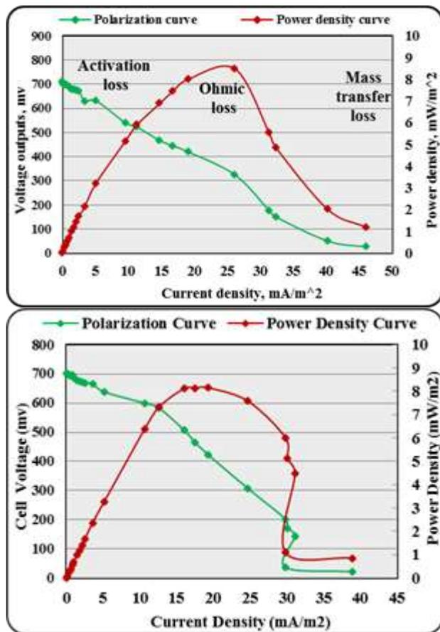
Figure 3. Polarization curves for; (A) MFC-CW1, (B) MFC-CW3
