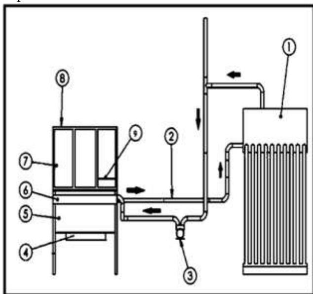
1. Tubular sun heater\ no. of tubes 10\ length of tube 180 cm\ tube diameter 6.3.
