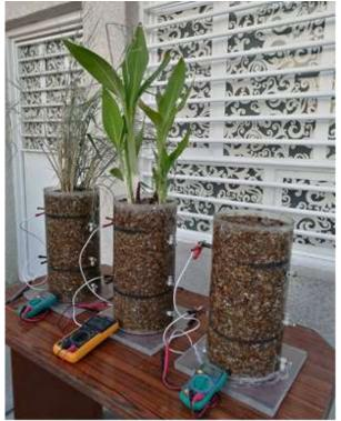
Plate 1. Photo of the MFC-CW systems Experimental procedure
